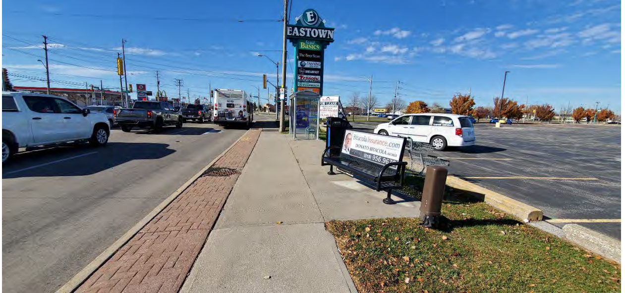
Figure 13 Example of a Near-Side Bus Stop
