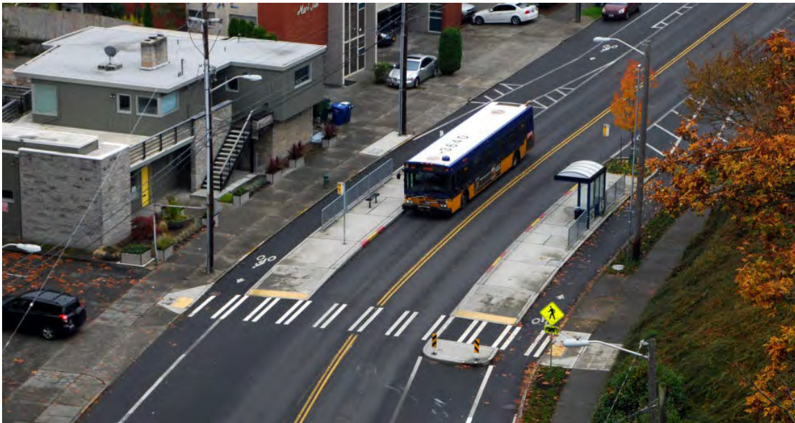
Figure 49 Side-Boarding Island Bus Stop Example
